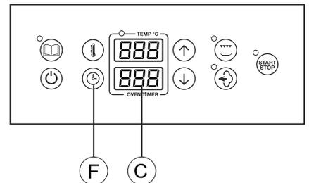
For an unlimited functioning of the oven (infinite time), press the button on the side, when the display shows value 0. The display will then show - - -.
