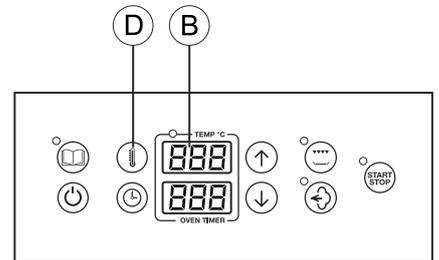
Press again temperature button (D) to store the new value for the cooking. The led stops flashing.
