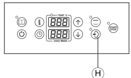
Press again humidification button to switch off the flashing led and store the new value for the cooking.
