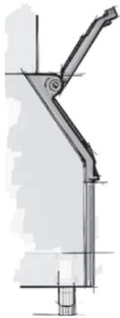
Slope front bins. Insulated, inside finished with rounded corners, for daily turnover of ice. Easy to clean and maintain with removable gaskets. The reinforced hinges provide enhanced durability. The slope front makes access to ice as easy as possible.
