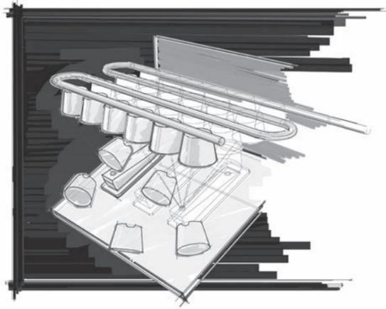
Horizontal ice evaporator and spray-system technology
